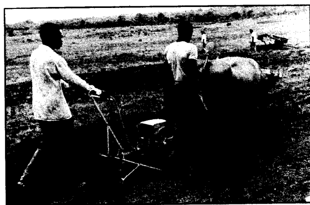
Fig 4.14 Planting upland rice with a Super Eco seeder
