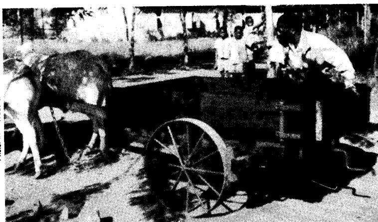
Photo 1: Wananchi ox cart, with steel wheels and block brakes
