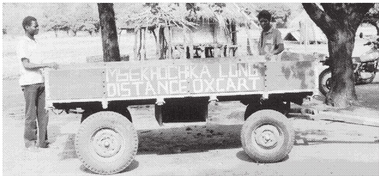
Figure 16. Four-wheeled ox cart used by the Msekhochika Project in Eastern Province as an alternative to a pickup vehicle.
