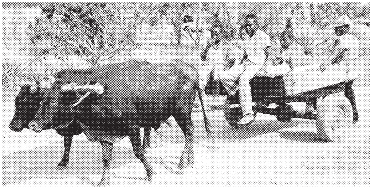
Figure 12. Ox cart made from an old axle in Lusaka Province.
